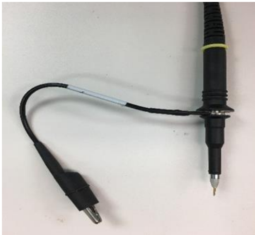
Figure 5: Passive probe with 3-inch group loop wire
