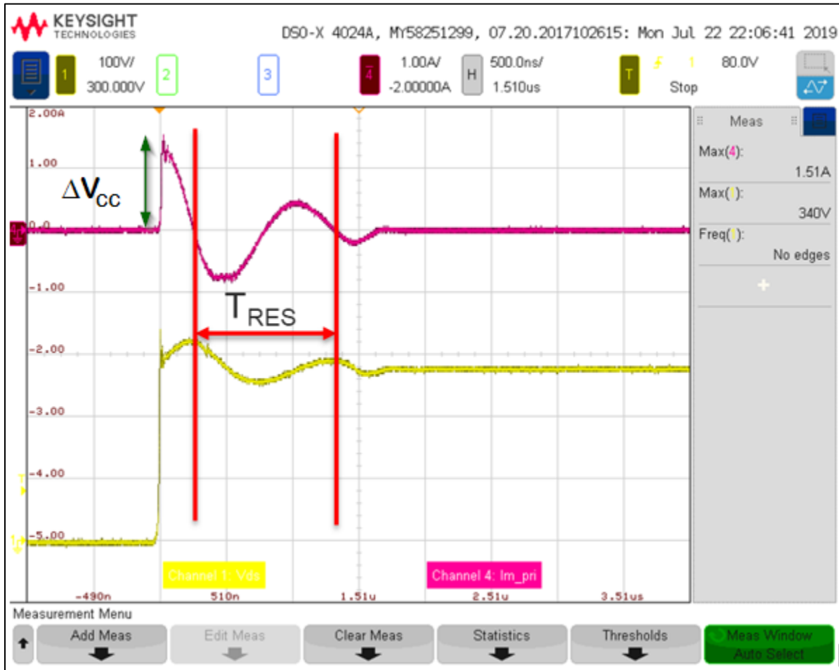
Figure 10: Typical primary MOSFET drain voltage and active clamp current with the active clamp resonant period highlighted
