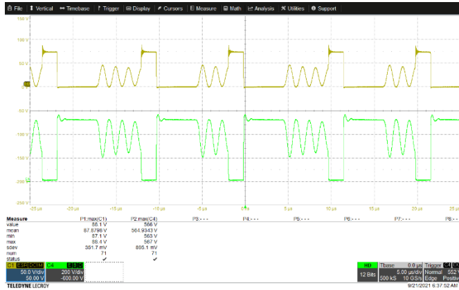
Vin=265 Vac, Vout=20 V, Iout=3.25 A, Vds_MAIN=567.0 V
