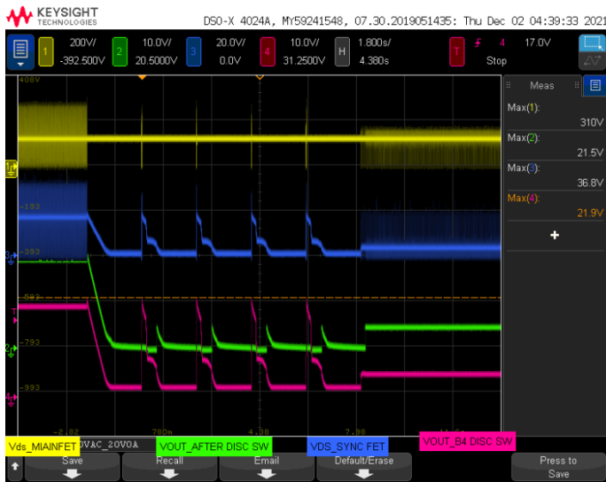
Vin=90 Vac, Vout=20 V, 0 A, Opto Shorted, VDS_max=310 V
