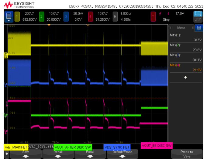
Vin=90 Vac, Vout=20 V, 1.65A, Opto Shorted, VDS_max=317 V
