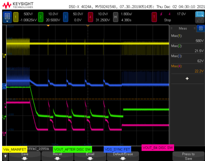
Vin=265 Vac, Vout=20 V, 0 A, Opto Shorted, VDS_max=580 V
