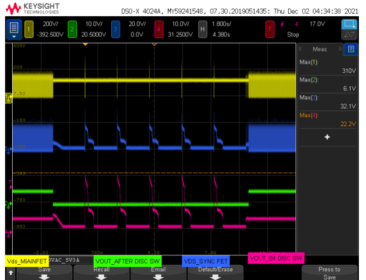
Vin=90 Vac, Vout=5 V, 3 A, Opto Shorted, VDS_max=310 V
