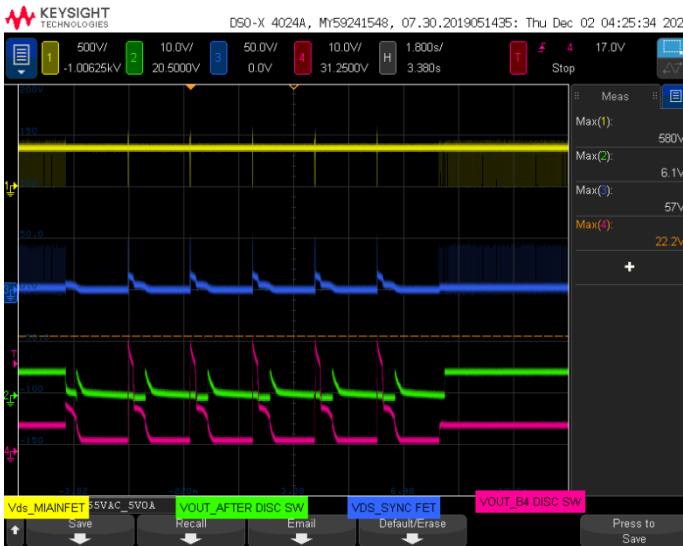
Vin=265 Vac, Vout=5 V, 0 A, Opto Shorted, VDS_max=580 V
