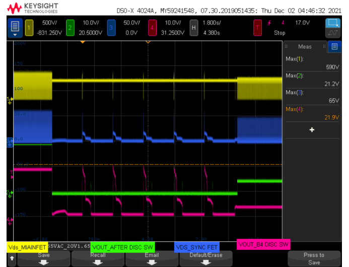
Vin=265 Vac, Vout=20 V, 1.65 A, Opto Shorted, VDS_max=590 V
