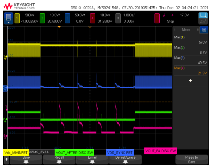
Vin=265 Vac, Vout=5 V, 3 A, Opto Shorted, VDS_max=570 V
