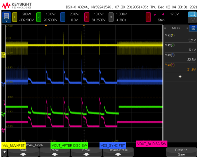
Vin=90 Vac, Vout=5 V, 0 A, Opto Shorted, VDS_max=321 V
