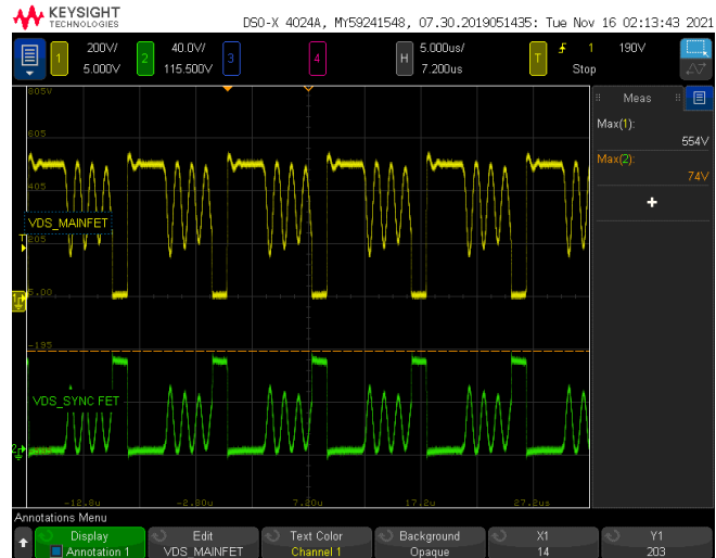
Vin=265 Vac, Vout=20 V, Iout=1.65 A, Vds_MAIN=554.0 V, Vds_SRFET=74 V
