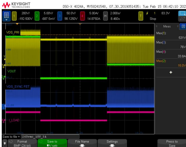
Vin=265 Vac, Vout=5 V, normal running then short, Recovery=5 V
