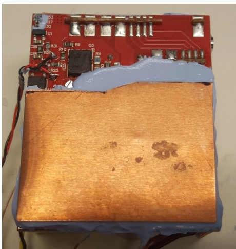
Metal heatsink on top of Bridge Rectifier, SZ1130 & Main FET
