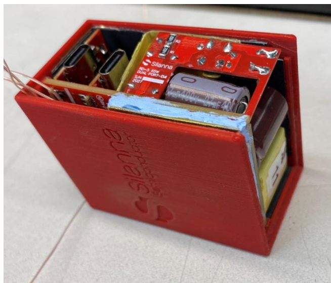
PCB assembly inside plastic case (L-shaped mating piece absent)
