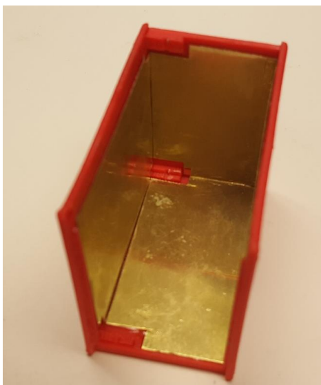
Heat spreader applied to case interior
