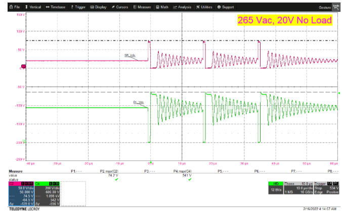
Vin=265 Vac, Vout=20 V, Iout=0 A, Vds_SRFET=74.2 V
