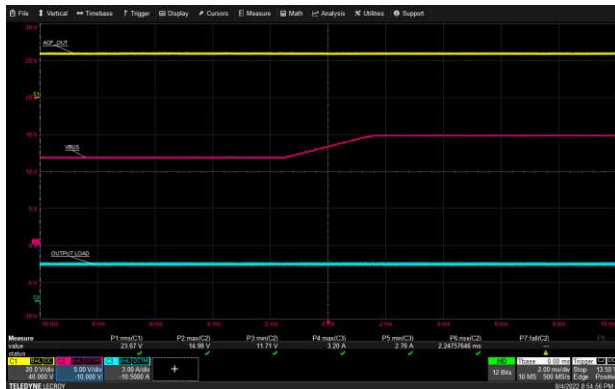
USB-C2 VBUS Transition: 90 Vac, 12 V to 15 V, 3 A Load
