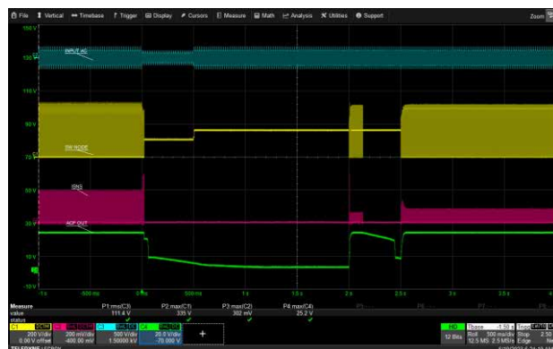
115 Vac to 75 Vac for 0.5 seconds, 20V/3.25A (USB-C1)
