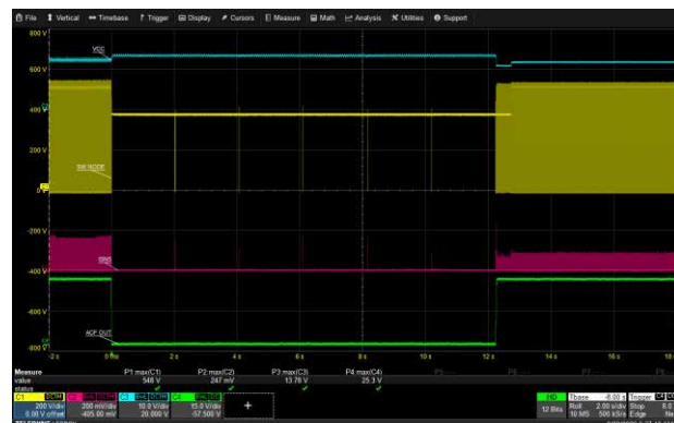
ACF_OUT Running Short Circuit: 265 Vac, 20V/3.25A USB-C1
