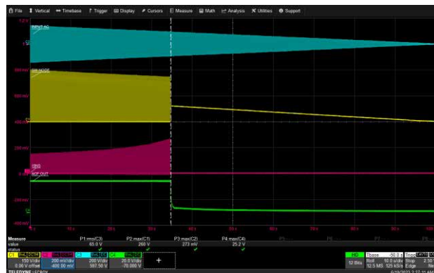
100 Vac to 0 Vac at 1 Vac/second, 15V/3A (USB-C1)
