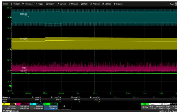
265 Vac to 290 Vac for 0.5 seconds, 20V/0A (USB-C1)
