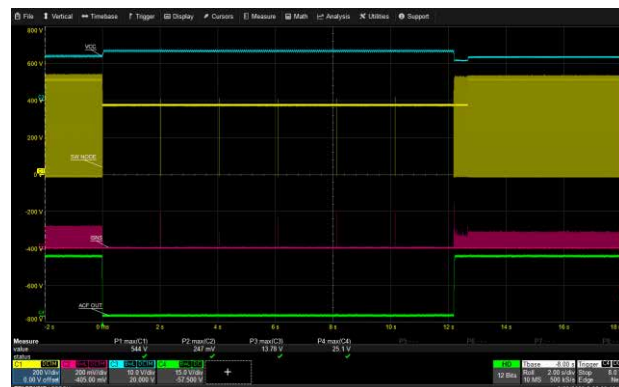
ACF_OUT Running Short Circuit: 265 Vac, 12V/3A USB-C1
