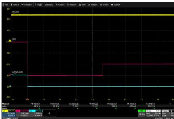
USB-C2 Over Voltage Protection: 90 Vac, 15V/3A
