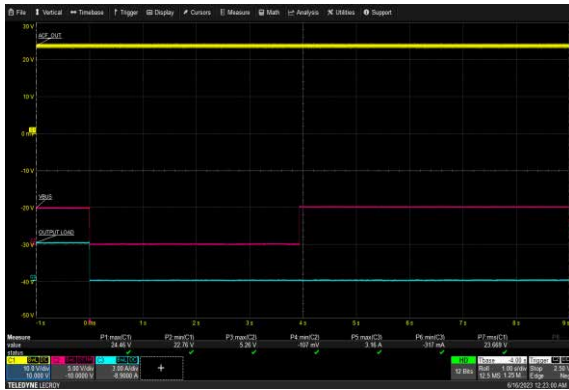
USB-C2 Over Voltage Protection: 90 Vac, 5V/3A
