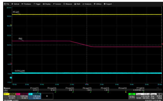
USB-A1 VBUS Transition: 265 Vac, 12 V to 9 V, 1.5 A Load
