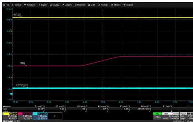
USB-A1 VBUS Transition: 90 Vac, 5 V to 9 V, 1.5 A Load
