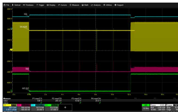
ACF_OUT Running Short Circuit: 265 Vac, 5V/3A USB-C1
