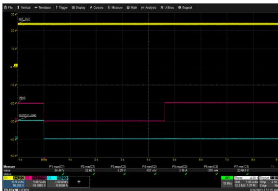
USB-C1 Over Voltage Protection: 90 Vac, 5V/3A
