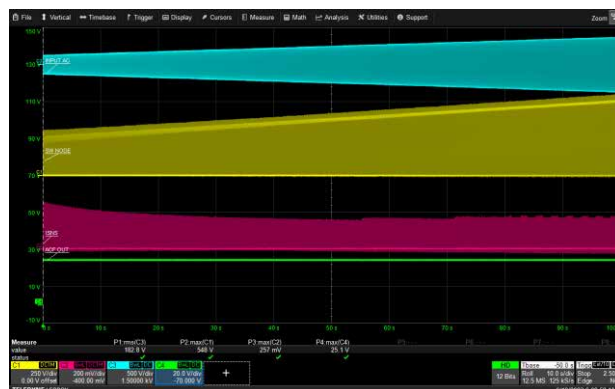
90 Vac to 290 Vac (at 1V/sec), 20V/3.25A (USB-C1)
