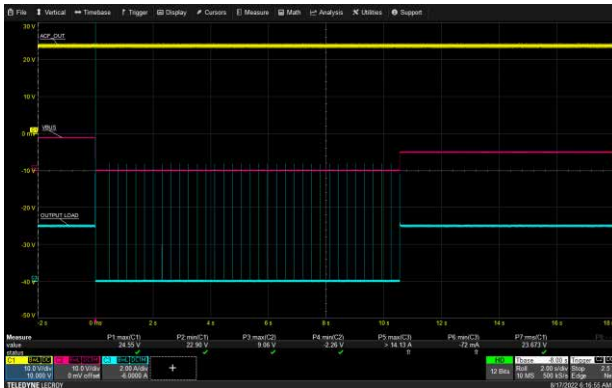
USB-C1 Short Circuit Protection: 90 Vac, 9V/3A
