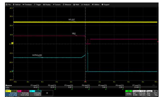
USB-C1 Over Current Protection: 265 Vac, 9 V
