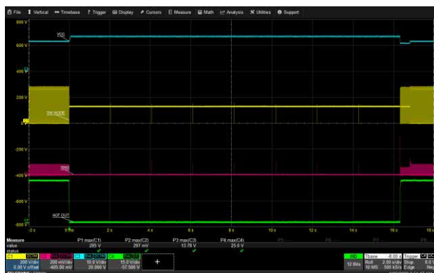
ACF_OUT Running Short Circuit: 90 Vac, 5V/3A USB-C1
