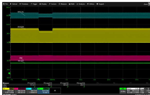
115 Vac to 75 Vac for 0.5 seconds, 9V/3A (USB-C1)
