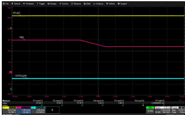
USB-C1 VBUS Transition: 90 Vac, 15 V to 12 V, 3 A Load
