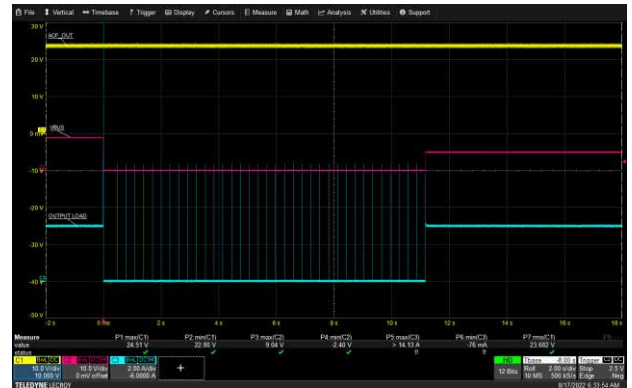
USB-C1 Short Circuit Protection: 265 Vac, 9V/3A
