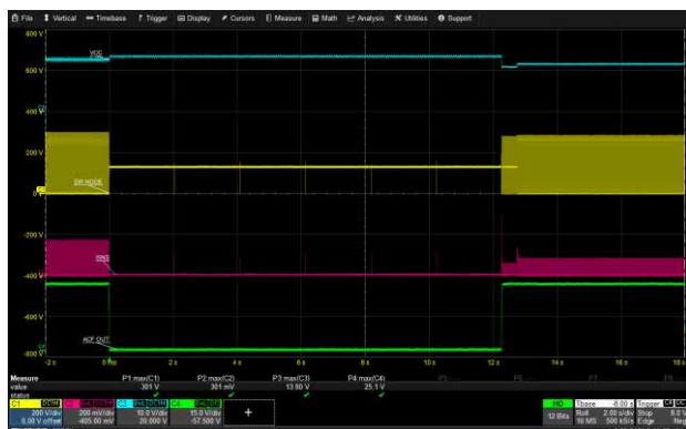
ACF_OUT Running Short Circuit: 90 Vac, 15V/3A USB-C1
