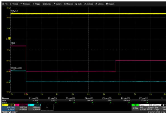
USB-C2 Over Voltage Protection: 90 Vac, 12V/3A
