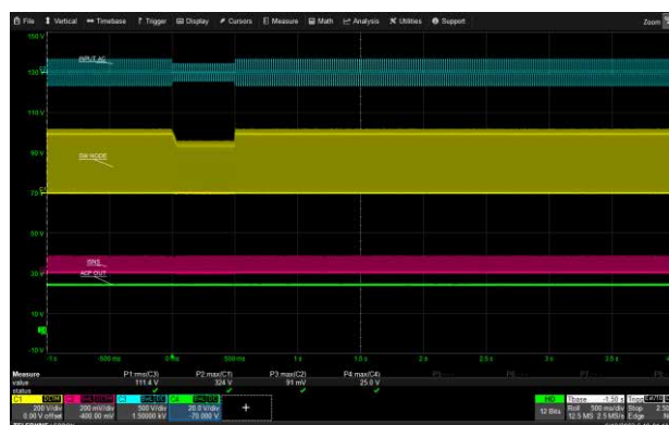
115 Vac to 75 Vac for 0.5 seconds, 5V/3A (USB-C1)
