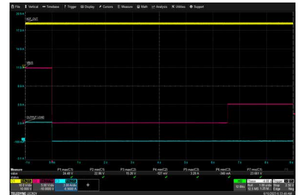
USB-C1 Over Voltage Protection: 90 Vac, 15V/3A
