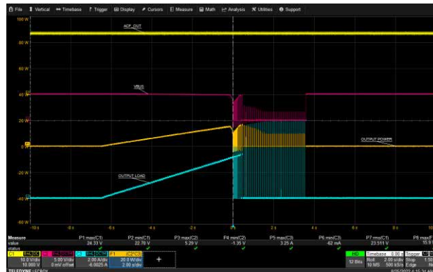
USB-A1 Over Current Protection: 265 Vac, 5 V
