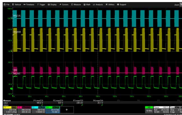
20 cycles of 0 Vac to 265 Vac, 5V/3A (USB-C1)
