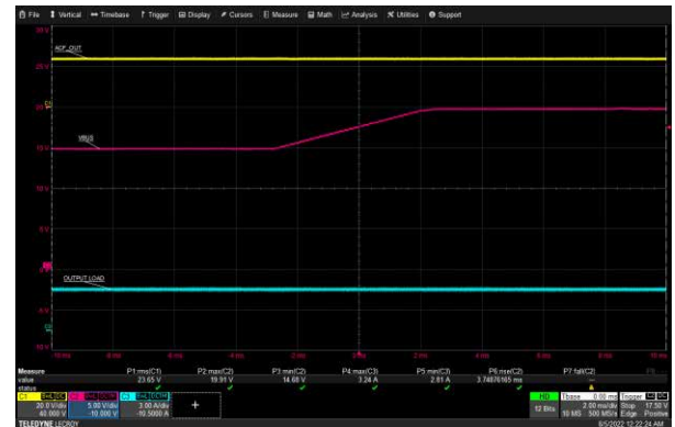
USB-C2 VBUS Transition: 265 Vac, 15 V to 20 V, 3 A Load
