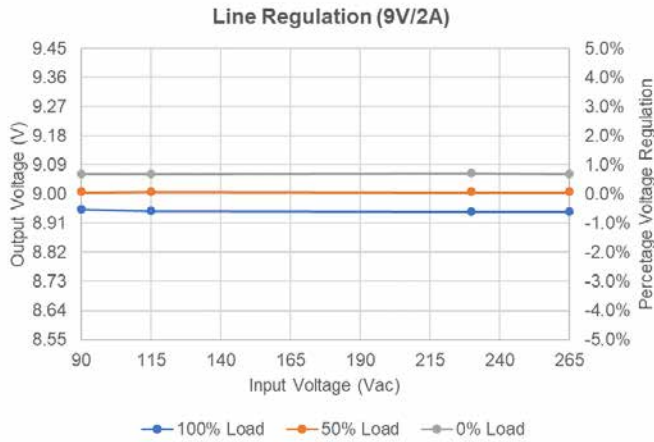
Slave USB-A1 Port Line and Load Regulation (9V/2A)
