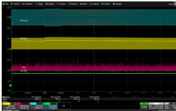
265 Vac to 290 Vac for 0.5 seconds, 12V/0A (USB-C1)
