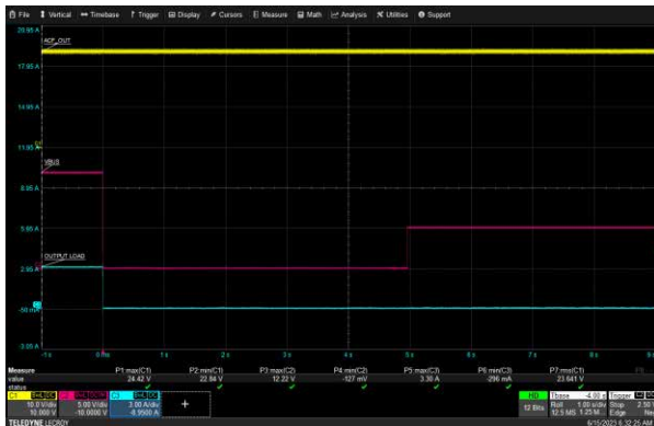
USB-C1 Over Voltage Protection: 90 Vac, 12V/3A
