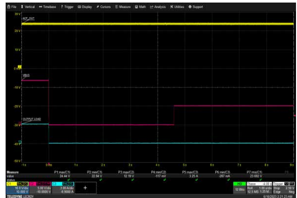
USB-C2 Over Voltage Protection: 265 Vac, 12V/3A
