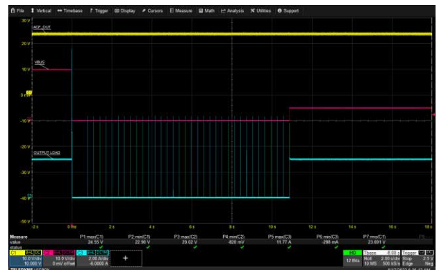
USB-C1 Short Circuit Protection: 265 Vac, 20V/3.25A
