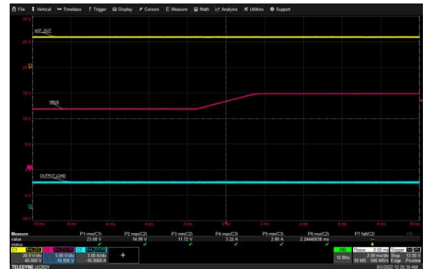
USB-C2 VBUS Transition: 265 Vac, 12 V to 15 V, 3 A Load
