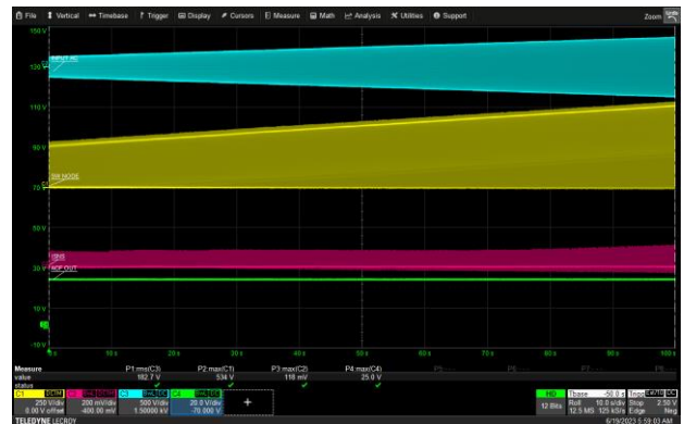
90 Vac to 290 Vac (at 1V/sec), 5V/3A (USB-C1)
