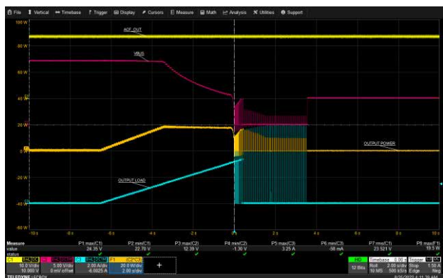
USB-A1 Over Current Protection: 90 Vac, 12 V
