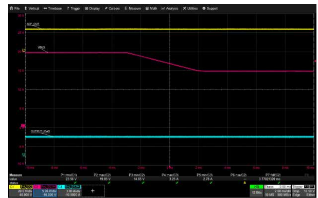
USB-C2 VBUS Transition: 90 Vac, 20 V to 15 V, 3 A Load
