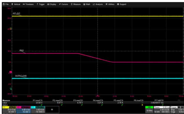
USB-C1 VBUS Transition: 90 Vac, 9 V to 5 V, 3 A Load
