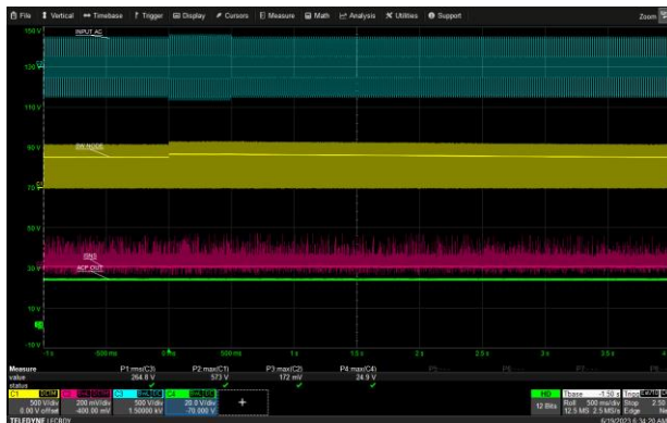
265 Vac to 290 Vac for 0.5 seconds, 9V/0A (USB-C1)
