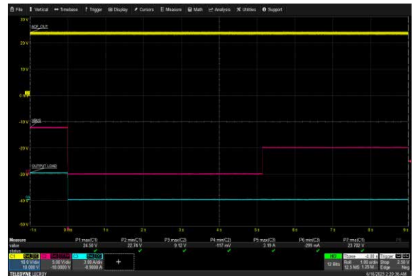
USB-C2 Over Voltage Protection: 265 Vac, 9V/3A
