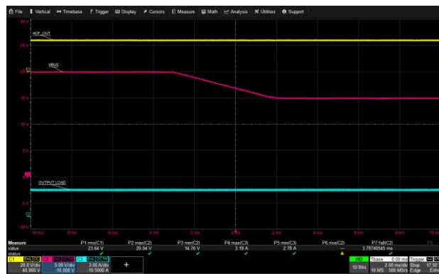
USB-C1 VBUS Transition: 265 Vac, 20 V to 15 V, 3 A Load
