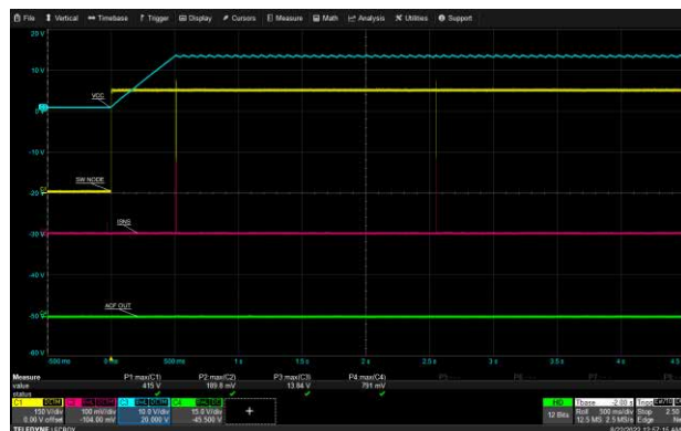
ACF_OUT Startup Short Circuit: 265 Vac
