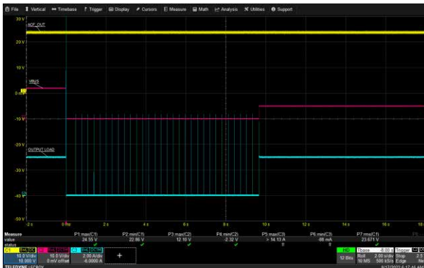
USB-C1 Short Circuit Protection: 90 Vac, 12V/3A
