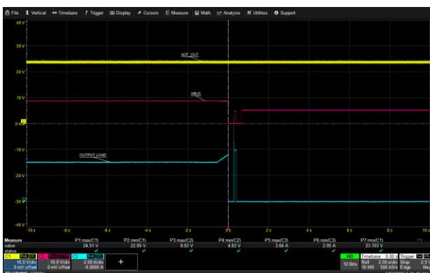
USB-C1 Over Current Protection: 90 Vac, 9 V
