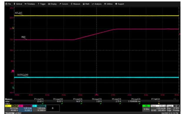
USB-C2 VBUS Transition: 90 Vac, 15 V to 20 V, 3 A Load
