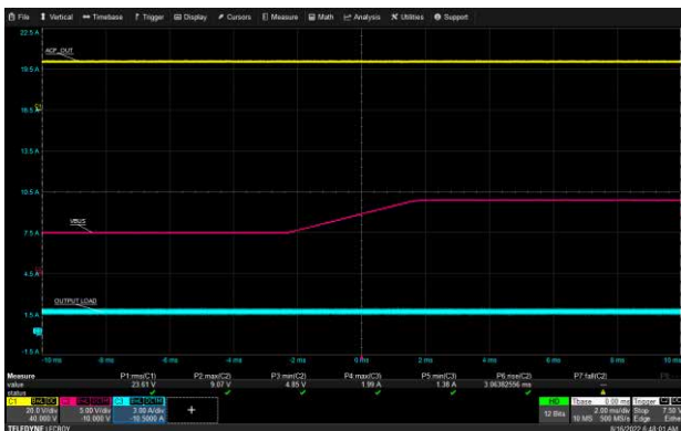
USB-A1 VBUS Transition: 265 Vac, 5 V to 9 V, 1.5 A Load
