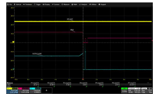
USB-C1 Over Current Protection: 265 Vac, 12 V
