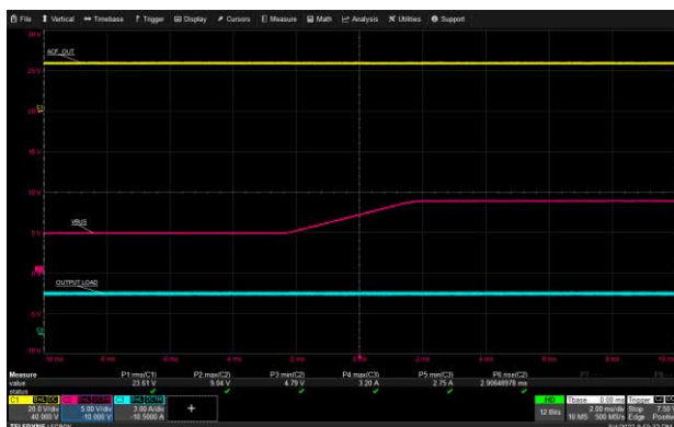
USB-C2 VBUS Transition: 90 Vac, 5 V to 9 V, 3 A Load
