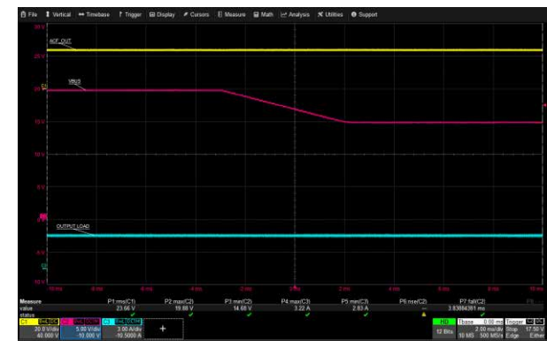
USB-C2 VBUS Transition: 265 Vac, 20 V to 15 V, 3 A Load
