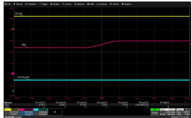
USB-C1 VBUS Transition: 265 Vac, 12 V to 15 V, 3 A Load
