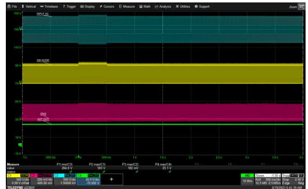
265 Vac to 290 Vac for 0.5 seconds, 20V/3.25A (USB-C1)
