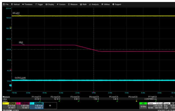
USB-A1 VBUS Transition: 90 Vac, 12 V to 9 V, 1.5 A Load
