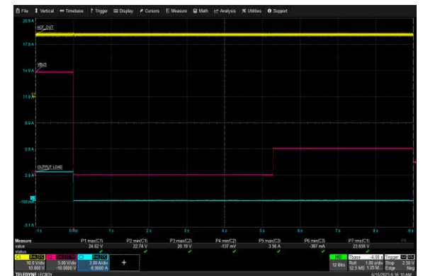
USB-C1 Over Voltage Protection: 90 Vac, 20V/3.25A
