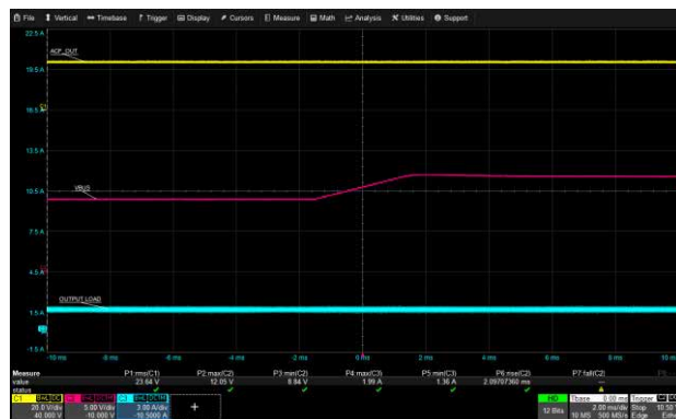
USB-A1 VBUS Transition: 265 Vac, 9 V to 12 V, 1.5 A Load
