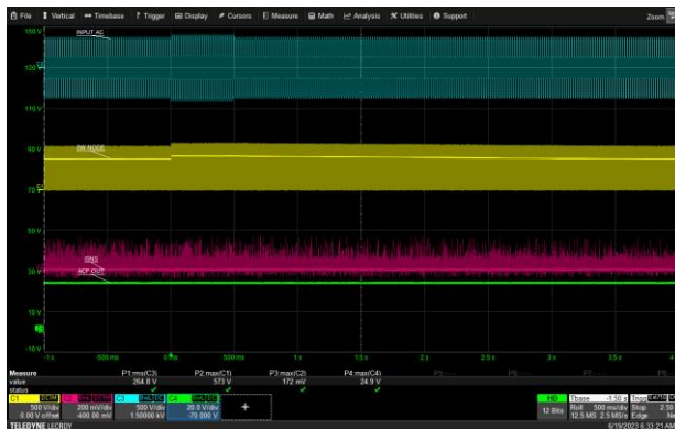
265 Vac to 290 Vac for 0.5 seconds, 5V/0A (USB-C1)
