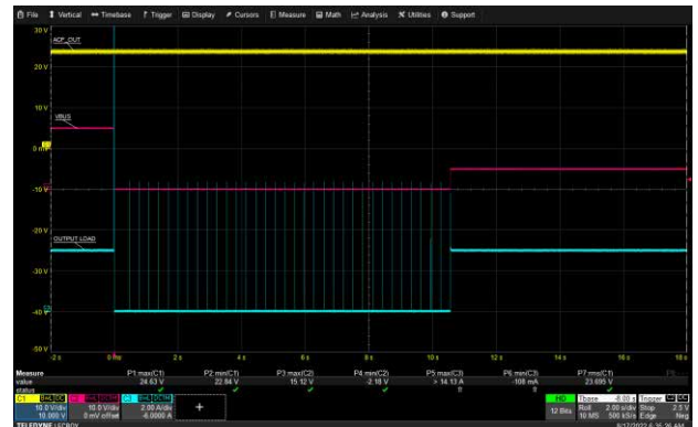
USB-C1 Short Circuit Protection: 265 Vac, 15V/3A
