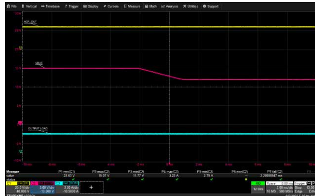
USB-C1 VBUS Transition: 265 Vac, 15 V to 12 V, 3 A Load
