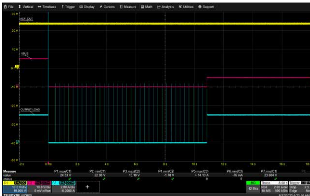
USB-C1 Short Circuit Protection: 90 Vac, 15V/3A
