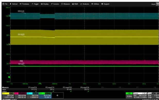
115 Vac to 75 Vac for 0.5 seconds, 12V/0A (USB-C1)
