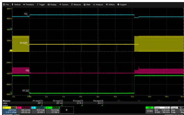
ACF_OUT Running Short Circuit: 90 Vac, 9V/3A USB-C1
