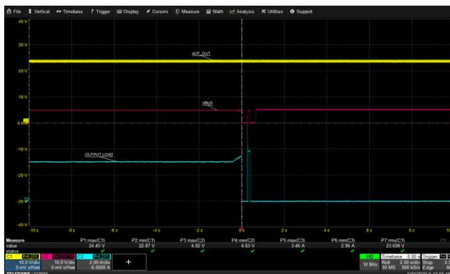
USB-C1 Over Current Protection: 265 Vac, 5 V
