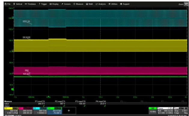
265 Vac to 290 Vac for 0.5 seconds, 12V/3A (USB-C1)
