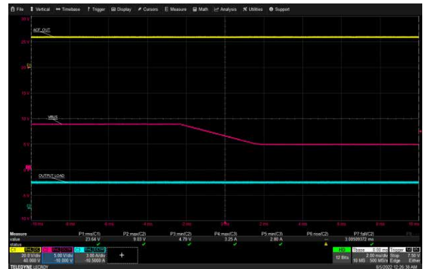
USB-C2 VBUS Transition: 265 Vac, 9 V to 5 V, 3 A Load
