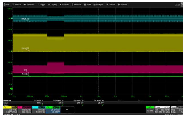
115 Vac to 75 Vac for 0.5 seconds, 15V/3A (USB-C1)
