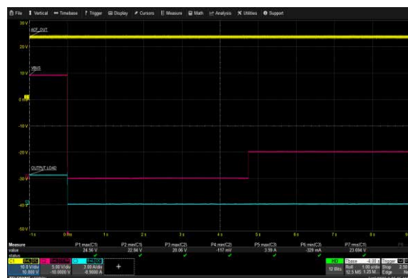
USB-C2 Over Voltage Protection: 265 Vac, 20V/3.25A
