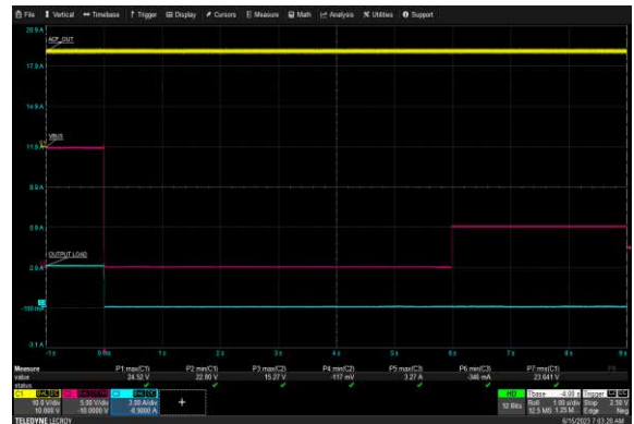
USB-C1 Over Voltage Protection: 265 Vac, 15V/3A
