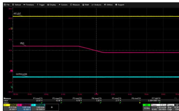
USB-C1 VBUS Transition: 265 Vac, 12 V to 9 V, 3 A Load
