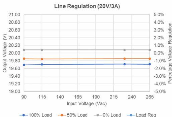
Slave USB-C2 Port Line and Load Regulation (20V/3.25A)
