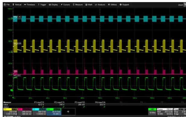
20 cycles of 0 Vac to 90 Vac, 5V/3A (USB-C1)
