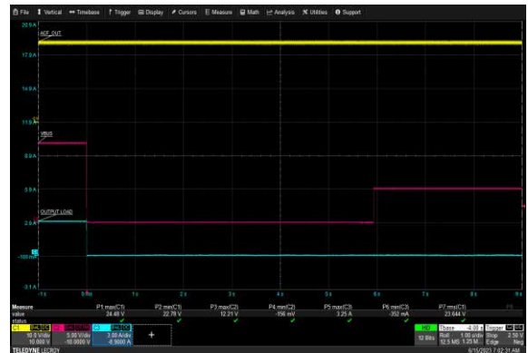
USB-C1 Over Voltage Protection: 265 Vac, 12V/3A
