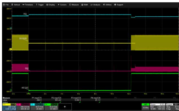
ACF_OUT Running Short Circuit: 90 Vac, 12V/3A USB-C1
