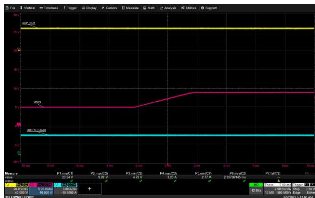
USB-C1 VBUS Transition: 90 Vac, 5 V to 9 V, 3 A Load
