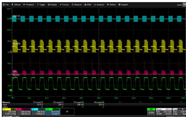
20 cycles of 0 Vac to 90 Vac, 5V/0A (USB-C1)
