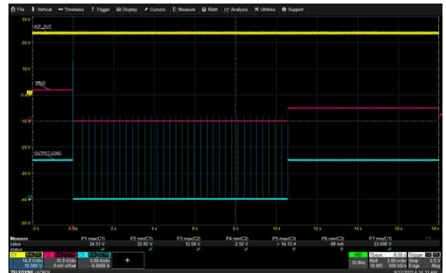
USB-C1 Short Circuit Protection: 265 Vac, 12V/3A
