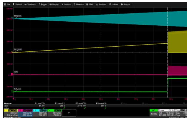
0 Vac to 100 Vac at 1 Vac/second, 5V/3A (USB-C1)
