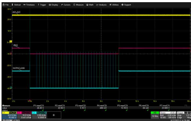
USB-C1 Short Circuit Protection: 90 Vac, 5V/3A
