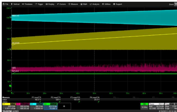
90 Vac to 290 Vac (at 1V/sec), 5V/0A (USB-C1)
