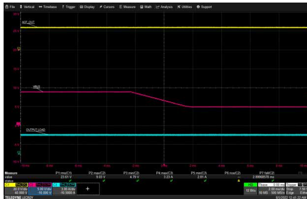
USB-C2 VBUS Transition: 90 Vac, 9 V to 5 V, 3 A Load
