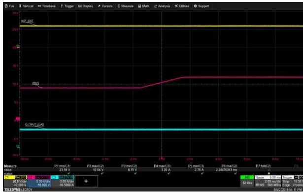
USB-C2 VBUS Transition: 90 Vac, 9 V to 12 V, 3 A Load
