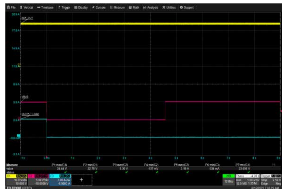
USB-C1 Over Voltage Protection: 265 Vac, 5V/3A
