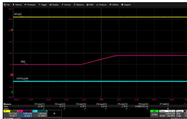
USB-C1 VBUS Transition: 265 Vac, 5 V to 9 V, 3 A Load
