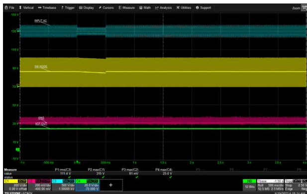
115 Vac to 75 Vac for 0.5 seconds, 15V/0A (USB-C1)
