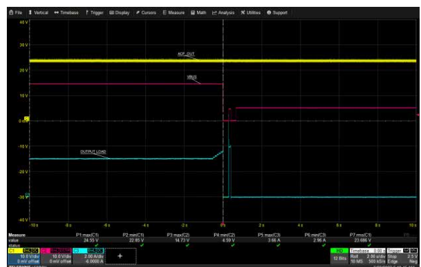
USB-C1 Over Current Protection: 90 Vac, 15 V
