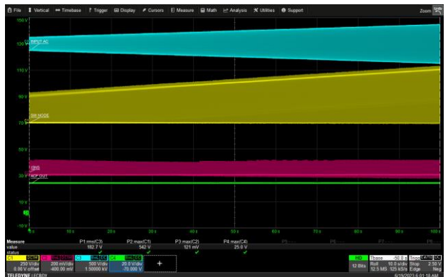
90 Vac to 290 Vac (at 1V/sec), 9V/3A (USB-C1)
