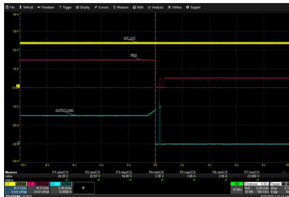
USB-C2 Over Current Protection: 265 Vac, 15 V
