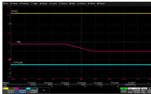
USB-C1 VBUS Transition: 265 Vac, 9 V to 5 V, 3 A Load
