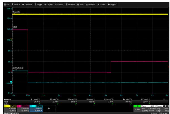
USB-C1 Over Voltage Protection: 265 Vac, 20V/3.25A
