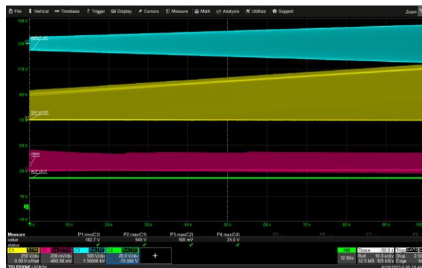
90 Vac to 290 Vac (at 1V/sec), 15V/3A (USB-C1)
