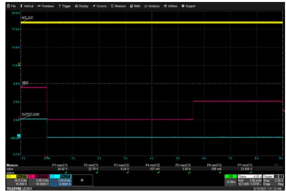
USB-C1 Over Voltage Protection: 265 Vac, 9V/3A
