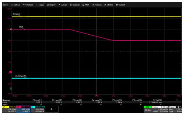
USB-C1 VBUS Transition: 90 Vac, 20 V to 15 V, 3 A Load
