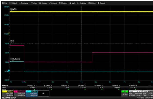
USB-C1 Over Voltage Protection: 90 Vac, 9V/3A
