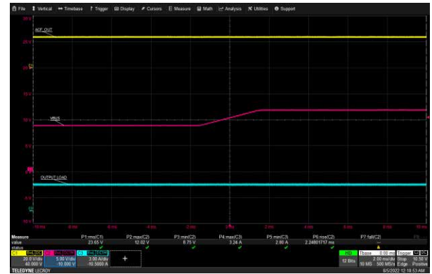
USB-C2 VBUS Transition: 265 Vac, 9 V to 12 V, 3 A Load
