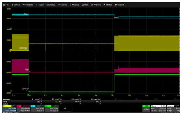
ACF_OUT Running Short Circuit: 90 Vac, 20V/3.25A USB-C1
