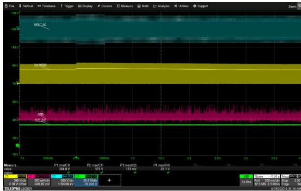
265 Vac to 290 Vac for 0.5 seconds, 15V/0A (USB-C1)
