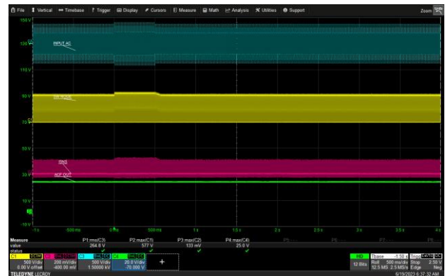
265 Vac to 290 Vac for 0.5 seconds, 5V/3A (USB-C1)
