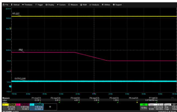
USB-A1 VBUS Transition: 90 Vac, 9 V to 5 V, 1.5 A Load
