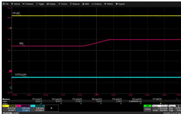
USB-C1 VBUS Transition: 90 Vac, 12 V to 15 V, 3 A Load
