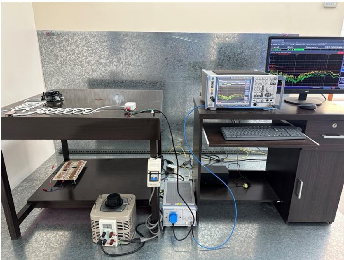
Figure 29. Conducted EMI Setup
