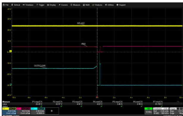
USB-C1 Over Current Protection: 90 Vac, 5 V
