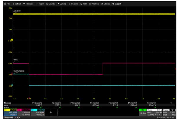
USB-C2 Over Voltage Protection: 265 Vac, 5V/3A
