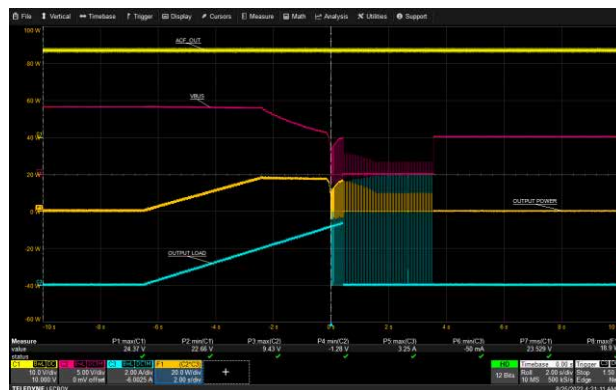
USB-A1 Over Current Protection: 265 Vac, 9 V
