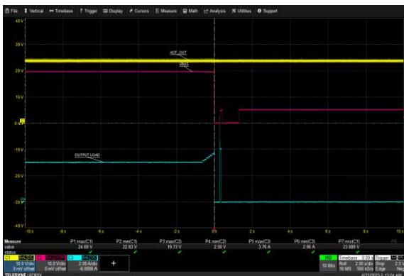
USB-C2 Over Current Protection: 90 Vac, 20 V
