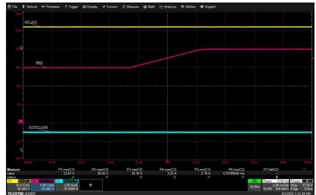
USB-C1 VBUS Transition: 265 Vac, 15 V to 20 V, 3 A Load
