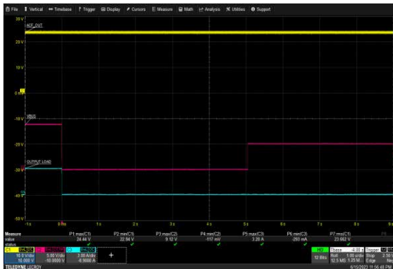
USB-C2 Over Voltage Protection: 90 Vac, 9V/3A
