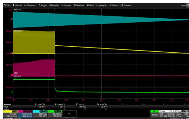
100 Vac to 0 Vac at 1 Vac/second, 20V/3.25A (USB-C1)
