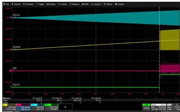
0 Vac to 100 Vac at 1 Vac/second, 5V/0A (USB-C1)
