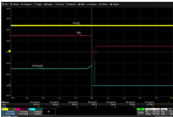
USB-C2 Over Current Protection: 90 Vac, 15 V
