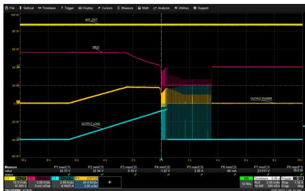
USB-A1 Over Current Protection: 90 Vac, 9 V
