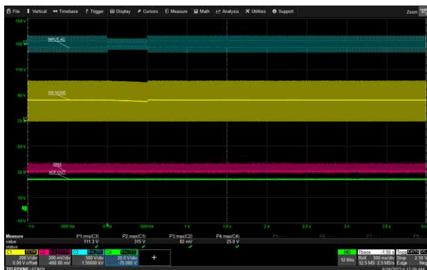
115 Vac to 75 Vac for 0.5 seconds, 9V/0A (USB-C1)
