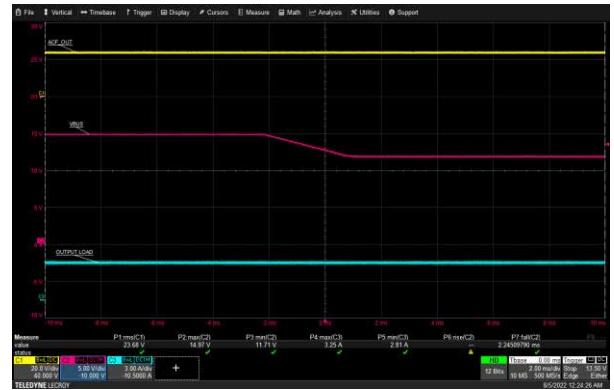
USB-C2 VBUS Transition: 265 Vac, 15 V to 12 V, 3 A Load
