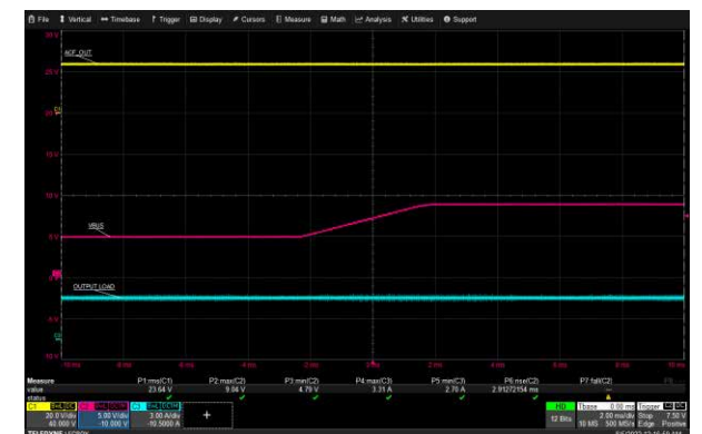
USB-C2 VBUS Transition: 265 Vac, 5 V to 9 V, 3 A Load
