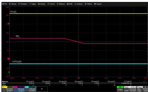
USB-C1 VBUS Transition: 90 Vac, 12 V to 9 V, 3 A Load
