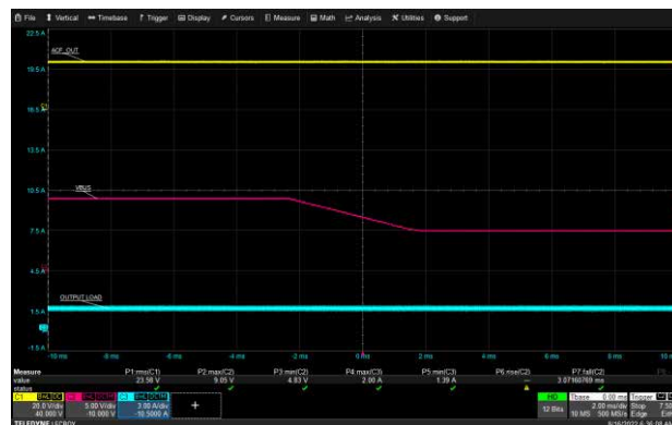
USB-A1 VBUS Transition: 265 Vac, 9 V to 5 V, 1.5 A Load
