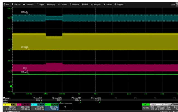
115 Vac to 75 Vac for 0.5 seconds, 12V/3A (USB-C1)
