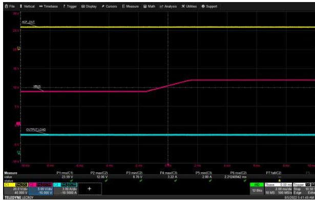
USB-C1 VBUS Transition: 90 Vac, 9 V to 12 V, 3 A Load
