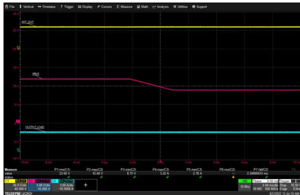
USB-C2 VBUS Transition: 90 Vac, 12 V to 9 V, 3 A Load
