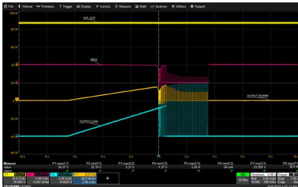
USB-A1 Over Current Protection: 90 Vac, 5 V
