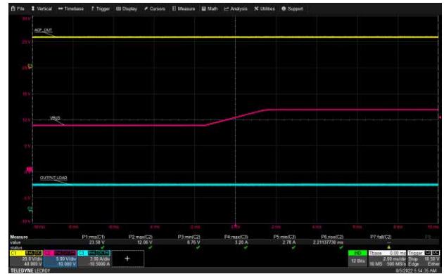
USB-C1 VBUS Transition: 265 Vac, 9 V to 12 V, 3 A Load
