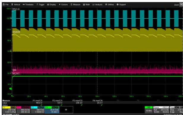
20 cycles of 0 Vac to 265 Vac, 5V/0A (USB-C1)
