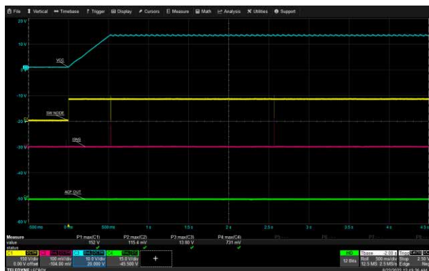
ACF_OUT Startup Short Circuit: 90 Vac
