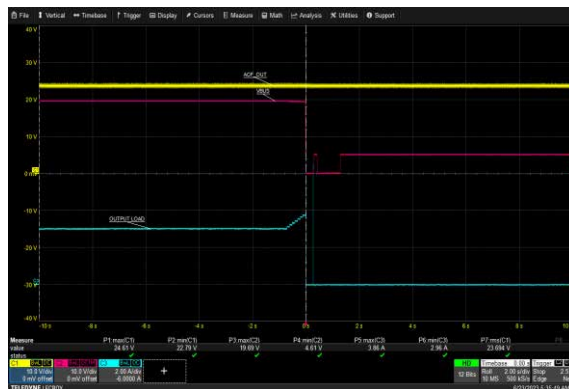
USB-C2 Over Current Protection: 265 Vac, 20 V
