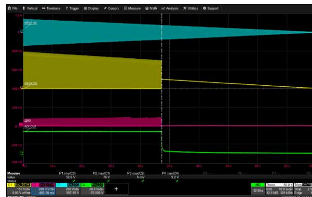
100 Vac to 0 Vac at 1 Vac/second, 5V/3A (USB-C1)
