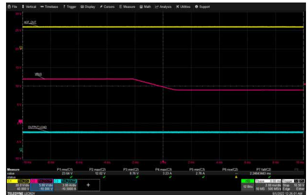
USB-C2 VBUS Transition: 265 Vac, 12 V to 9 V, 3 A Load
