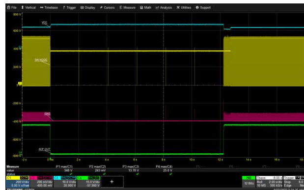
ACF_OUT Running Short Circuit: 265 Vac, 9V/3A USB-C1
