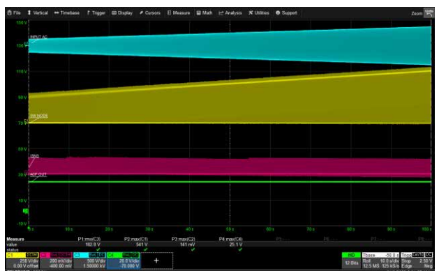
90 Vac to 290 Vac (at 1V/sec), 12V/3A (USB-C1)
