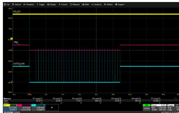
USB-C1 Short Circuit Protection: 265 Vac, 5V/3A
