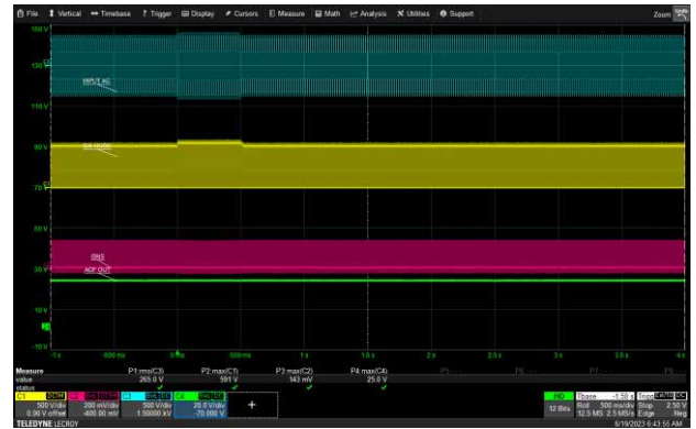
265 Vac to 290 Vac for 0.5 seconds, 15V/3A (USB-C1)
