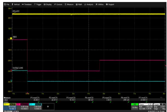
USB-C2 Over Voltage Protection: 265 Vac, 15V/3A
