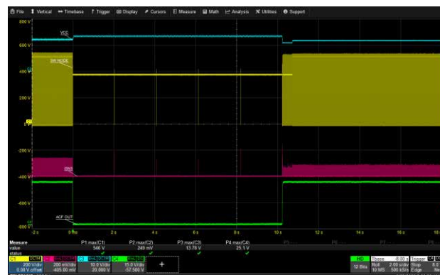
ACF_OUT Running Short Circuit: 265 Vac, 15V/3A USB-C1
