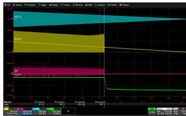
100 Vac to 0 Vac at 1 Vac/second, 5V/0A (USB-C1)
