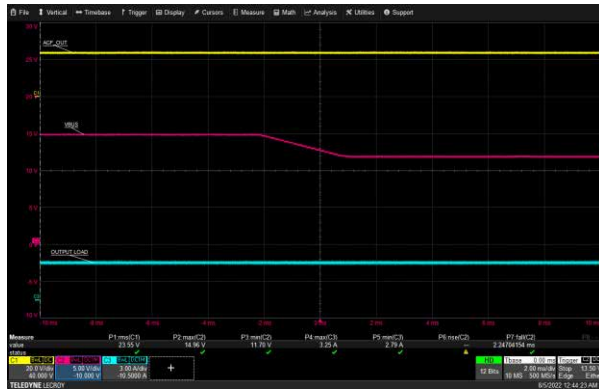
USB-C2 VBUS Transition: 90 Vac, 15 V to 12 V, 3 A Load
