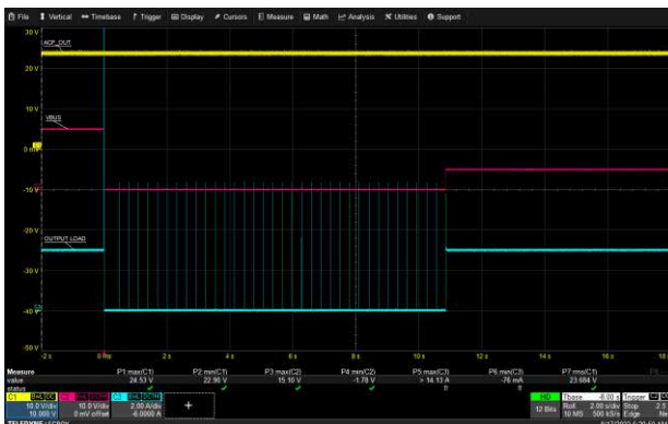
USB-C1 Short Circuit Protection: 90 Vac, 20V/3.25A
