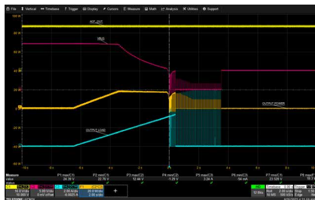
USB-A1 Over Current Protection: 265 Vac, 12 V
