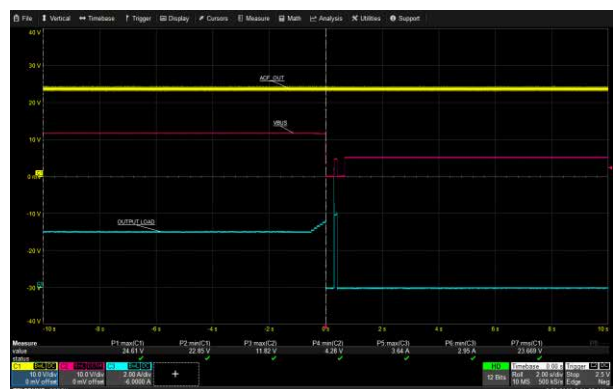
USB-C1 Over Current Protection: 90 Vac, 12 V
