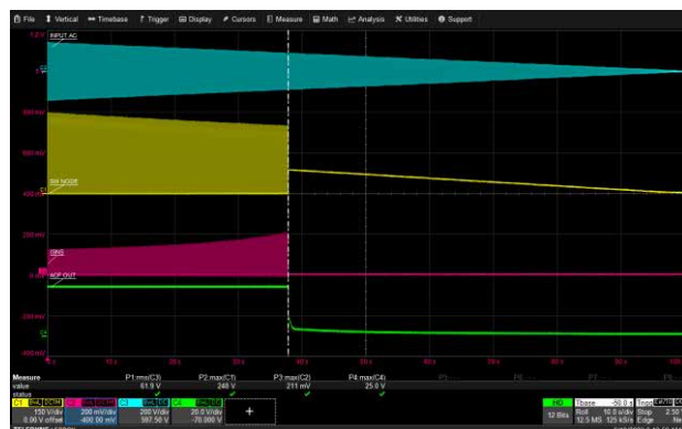
100 Vac to 0 Vac at 1 Vac/second, 12V/3A (USB-C1)
