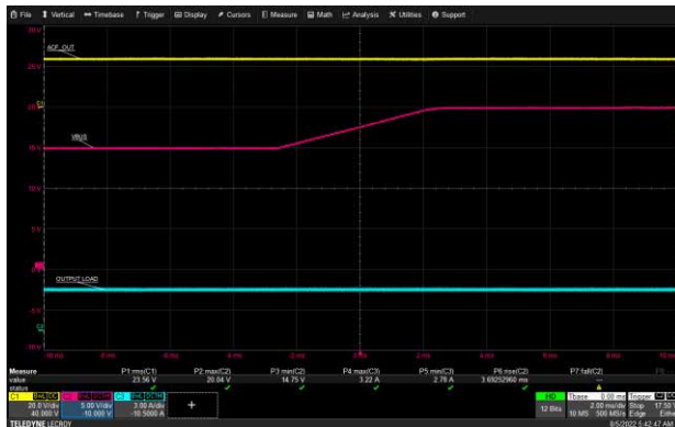
USB-C1 VBUS Transition: 90 Vac, 15 V to 20 V, 3 A Load
