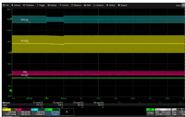
115 Vac to 75 Vac for 0.5 seconds, 20V/0A (USB-C1)
