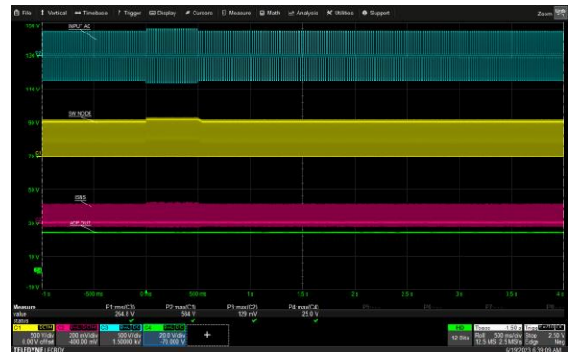
265 Vac to 290 Vac for 0.5 seconds, 9V/3A (USB-C1)
