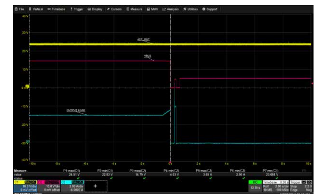
USB-C1 Over Current Protection: 265 Vac, 15 V
