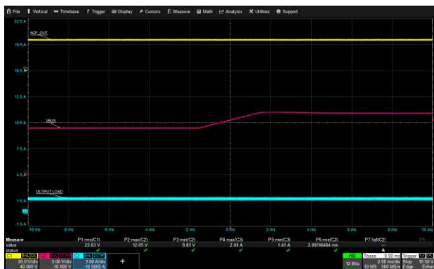
USB-A1 VBUS Transition: 90 Vac, 9 V to 12 V, 1.5 A Load
